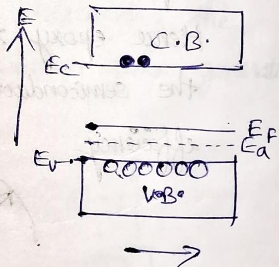
As temperature increases, thermally generated electron-hole pairs increase in addition to the majority holes due to acceptors.
