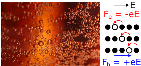
(a) Analogy for a hole: Bubbles (b) Drift motion of holes
