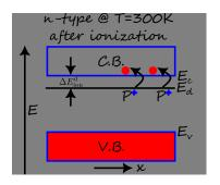
Upon ionization, the donor dopant releases free electron into the conduction band.
