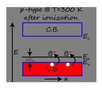
Upon ionization, the acceptor dopant accepts electron from valence band and creates a hole in the valence band.
