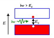
• In semiconductors, photon with energy greater than energy band gap  $E_g$ , it is absorbed and leads to generation of electron-hole pair.
